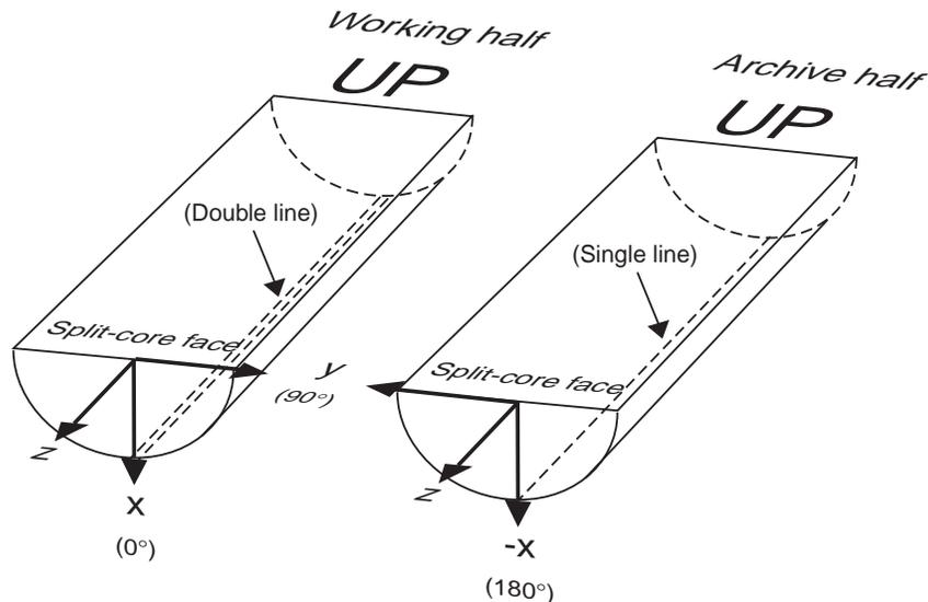
Figure 1—1 Core orientation conventions.
