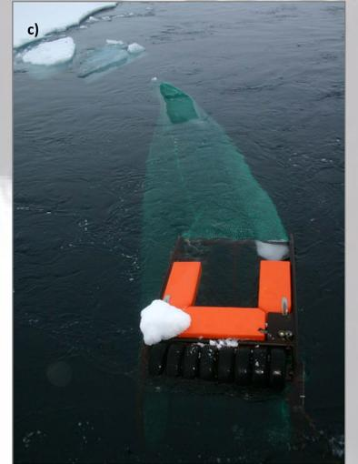
Fig.1 Surface and Under-Ice Trawl in Arctic Ocean (SUIT; van Franeker et al. 2009)
