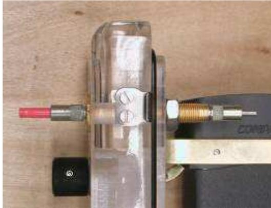
**Figure 3 Vacuum feed-through for optical cable.**
