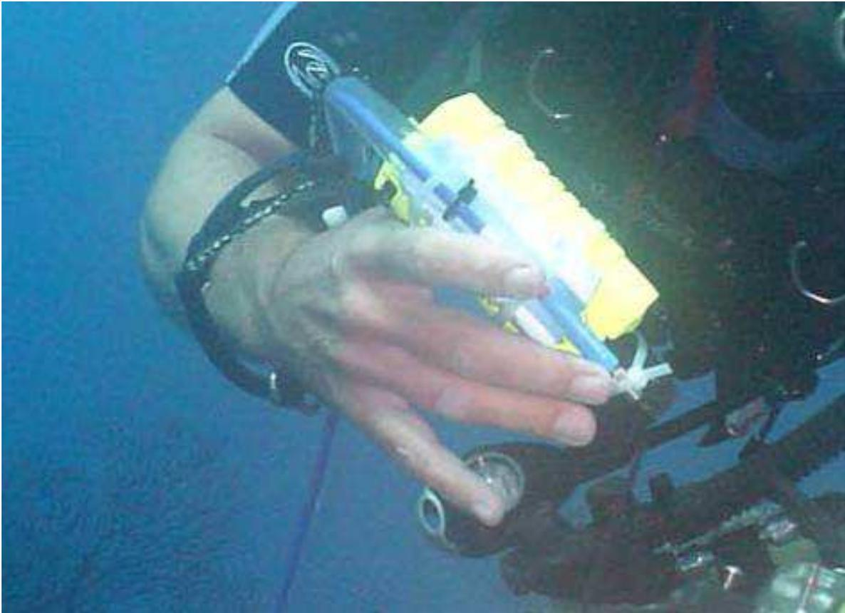
**Figure 12 Dive torch attached to fibre optic cable**
