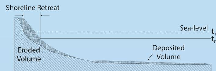
Fig. 3. Shoreline retreat resulting from sea-level rise, the Bruun rule. Note deposition on lower shoreface.
