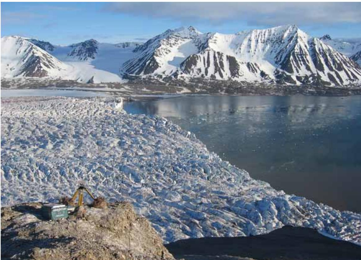
Fig. 2.4-11. Time-lapse cameras were used to monitor ice flux and calving on Kronebreen, Svalbard. (Photo: Monica Sund)
