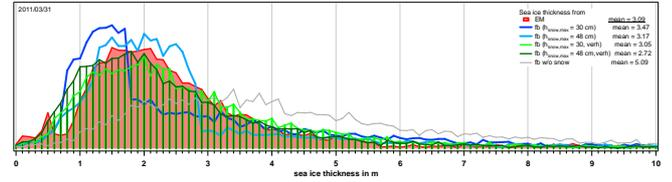
Sea ice thicknesses derived from freeboard measurements by
