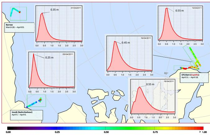
Flight tracks of laser scanner measurements in the Beaufort and Lincoln Sea. Colored dots indicate mean sea ice freeboard, histograms show freeboard distribution of the respective regions.
