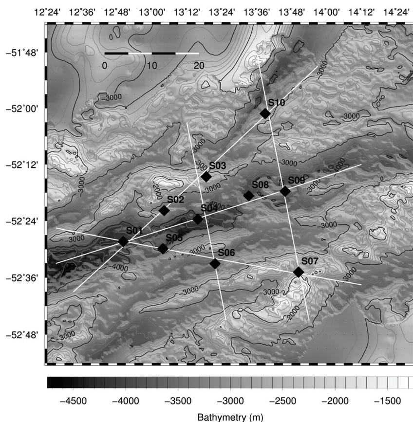
Fig. 1.2.1: Survey area at the Oblique Supersegment of the SWIR. Black diamonds indicate position of OBS S01-S10. White lines are planned airgun profiles. Distance scale is in kilometer. Bathymetry data as published in Dick *et al.* (2003)
