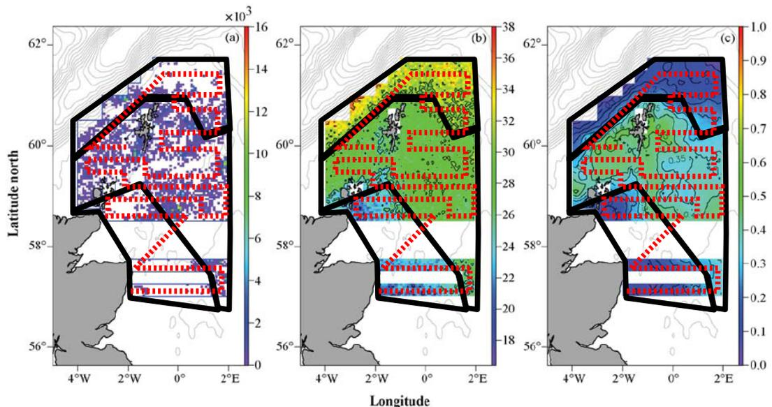
Figure 2. Data fields required for acoustic biomass assessment of a given species: a) total fish acoustic backscatter; b) species mean length; c) proportion by species and/or size class. Red dotted line: ship track; black lines: homogeneous regions boundaries. (Adapted from Woillez et al., 2009).
