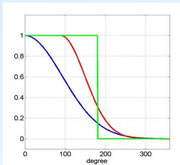
The **cutoff filter** up d/o 180 compared with the **Gauss filter** and the **Butterworth filter** referring to the same threshold.
