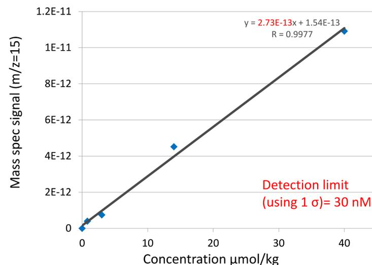
Methane calibration curves with German frit 1200 (32.5% Porosity) (~1/8" diam)
