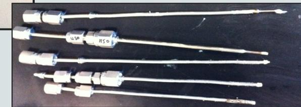
Our two research groups used metallic porous frits to mechanically support PDMS membranes, allowing the deployment of the UMSs to ocean depths of 2000 meters
