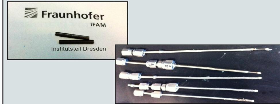
Our two research groups used metallic porous frits to mechanically support PDMS membranes, allowing the deployment of the UMSs to ocean depths of 2000 meters
