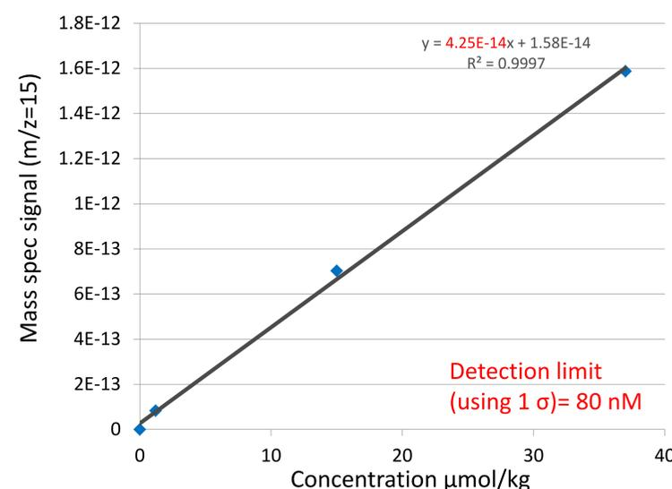
Methane calibration curves with German frit 1200 (48.3% Porosity) (~1/8" diam)
