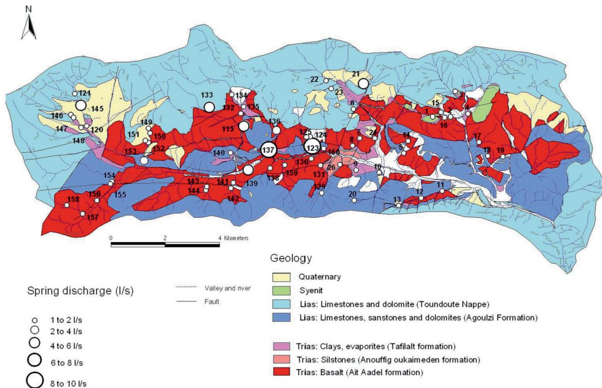
Fig. 1: Detailed geological map of the Assif-n-Ait Ahmed Catchment with mean spring discharge quantities (Cappy, 2006).
