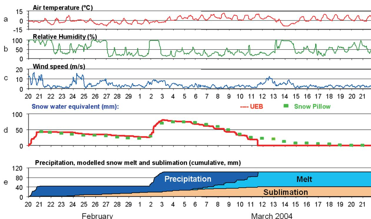
**Fig.2:** Measurements at the Tounza station (a, b, c: weather data from the automatic weather station, d: snow water equivalent calculated from snow weight on a snow pillow) and e: UEB-modelled snow ablation processes (melt and sublimation; precipitation was measured).
