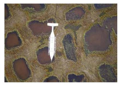
Fig. 3.4: The helicopter towed sensor "Helipod" during measurement of turbulent heat and  ${\rm CO}_2$  fluxes over the Siberian Lena Delta. (Photo: Torsten Sachs, GFZ)
