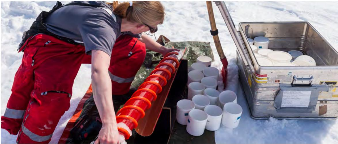
**Figure 91:** Preparation of sea-ice core for segmentation. Photo: Mario Hoppmann
