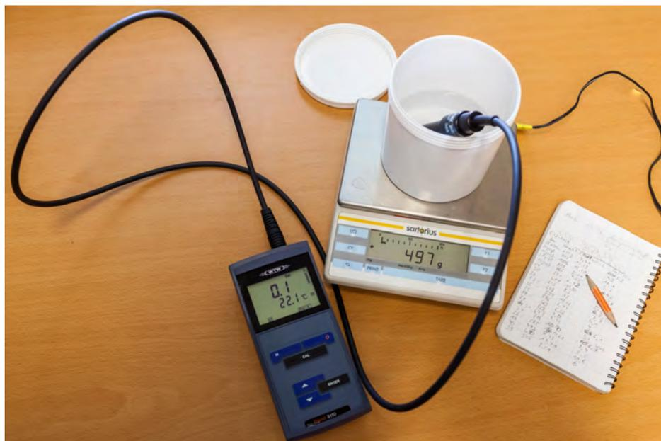
**Figure 93:** *WTW Cond3110* Conductivity-Meter. Photo: Mario Hoppmann
