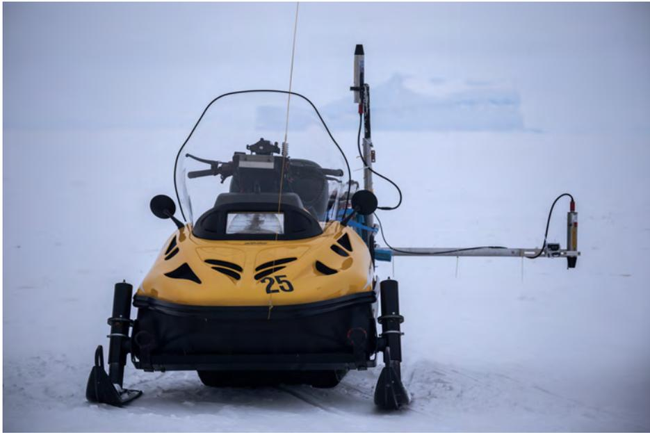
**Figure 56:** Two RAMSES sensors mounted on “Albedo skidoo”. The Zarges Box with the laptop and the generator are located on the back of the snowmobile. Photo: Mario Hoppmann
