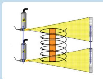
Figure 2: Sketch of the Helical-CT measurement method. Using a vertical feed during the rotation reduce the Feldkamp artifacts and allows measurements of theoretically arbitrary height.
