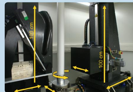
Figure 3: Detector (right) are equipped with climatic shielding (CFK, internal heater) and mounted on air puffed axes. An ice core piece of 1 m length is fixed on a rotation table seen in the CT laboratory. The ICE-CT manipulator system is based on 3 heavy granite quaders, X-Ray tube (left) and e middle, 6 additional axis can be driven (yellow arrows).
