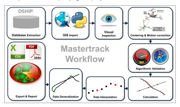
Figure 1: Workflow of master track data processing
