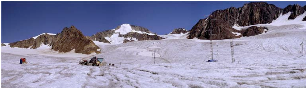
Figure 4: Measurement of energy balance components with the HyMEX-Station using Eddy-Correlation-method and a 9-m-profile-tower on Vernagtferner August 2000 at 2995 m a.s.l. At the left side the required mobile power station and two tents to shelter the data acquisition computers. (Panoramic Photo taken by M. Weber)
