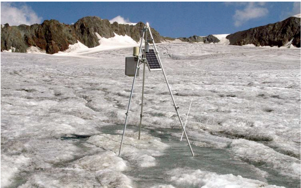
Figure 7: “On-glacier” ablation station, equipped with a sonic range sensor and a ventilated shielded Pt100-thermometer. (Photo taken in 2003 by M. Siebers).
