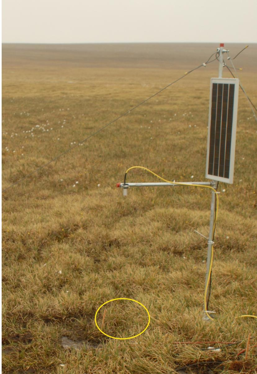
Figure 23: Station with Precision Infrared Temperature Sensor in a zone of wet sedge tundra in the Polar Bear Pass wetland area. The yellow circle indicates the field of view of the radiometer with about 0.28 m in diameter.
