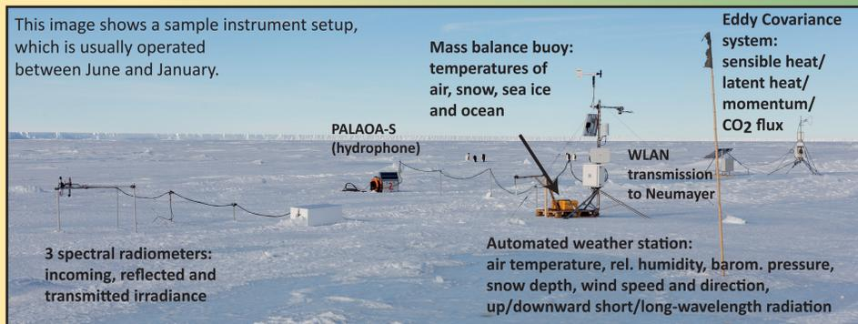
3 spectral radiometers: incoming, reflected and transmitted irradiance
