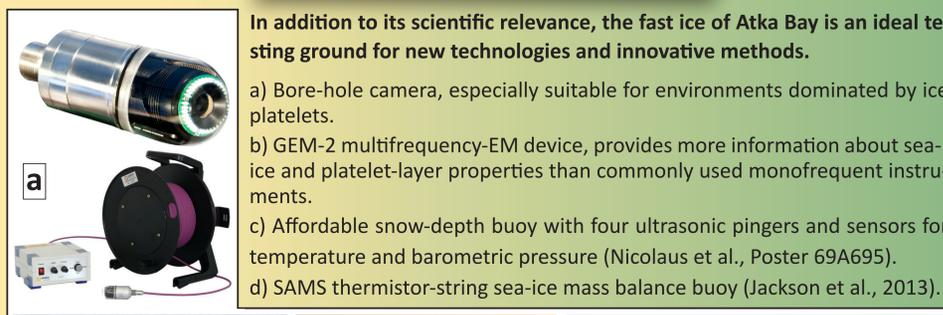
a) Bore-hole camera, especially suitable for environments dominated by ice platelets.
