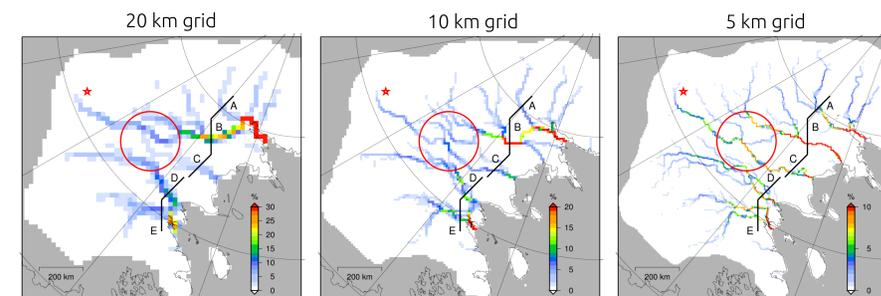
Fig. 5: Simulated basal water pathways at the Siple Coast for present-day bedrock elevation and ice thickness. The color scale shows the drainage in percent of the total catchment area and is truncated for a better visibility of the pathways, maximum values at the grounding line are 20 % (5 km), 31 % (10 km) and 42 % (20 km).
