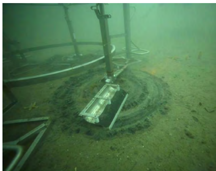
Above left: The Autonomous Sediment Disturber upon deployment at HAUSGARTEN off Svalbard. In the lower left corner push cores used for sampling by a remotely operated vehicle are visible. Image: MARUM at Bremen University and Thomas Soltwedel, AWI. Above right: The rotating plough-like unit disturbing sediments in a shallow water deployment to assess impacts on small sediment fauna and functions. Image: Thomas Soltwedel, AWI.
