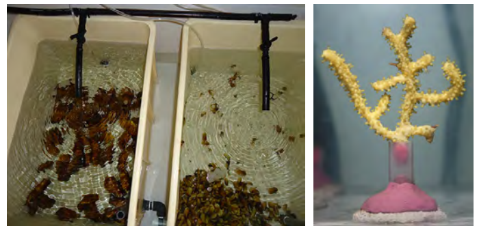
Above: The laboratory setup at LabHorta, designed to investigate the short-term impacts of sediment burial on the cold-water coral Dentomuricea sp. (top and bottom right) and the hydrothermal vent mussel Bathymodiolus azoricus (bottom left). Images courtesy IMAR/DoP-UAz.
