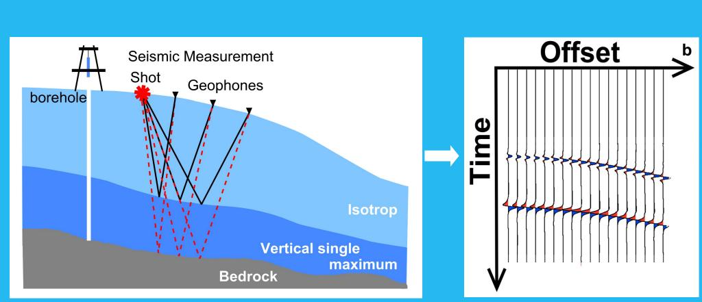
Fig. 1: (a) Sketch of seismic survey on ice with changing crystal orientation fabric (COF) over depth. (b) Reflections are expected form englacial and ice-bed boundary layers.
