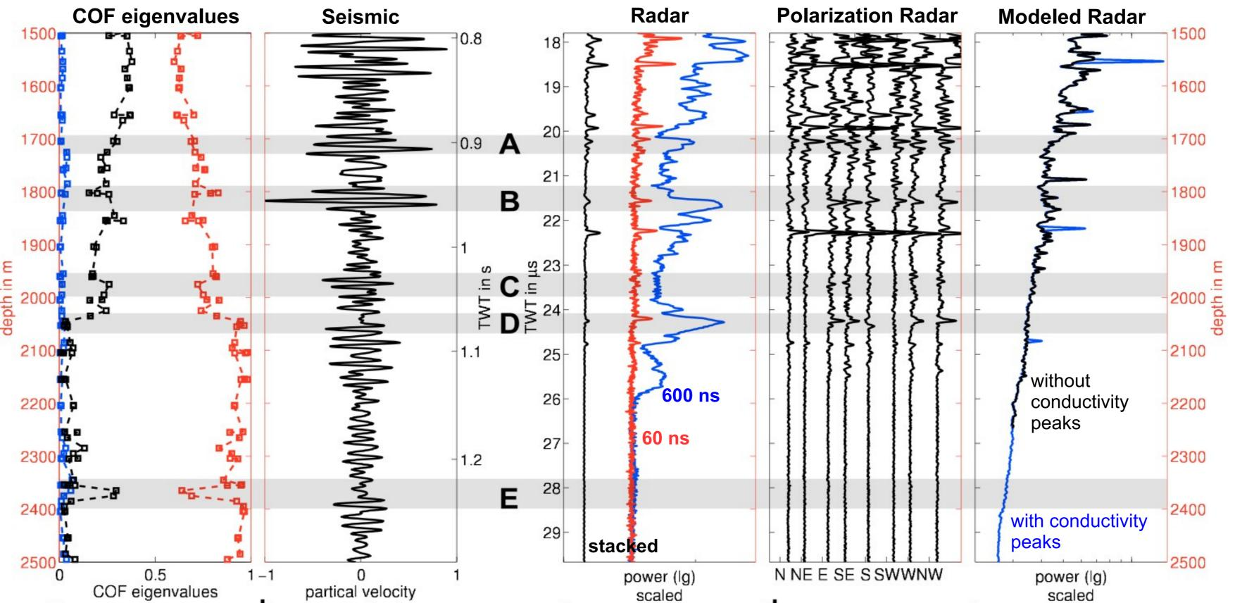
Fig. 6: (a) COF eigenvalues of EDML ice-core, (b) seismic trace, stack of 60 traces to enhance signal-toradar traces, in blue 600 ns pulse (023150), in red 60 ns pulse (022150), in black stack of all traces of the survey 033042 (60 ns pulse), (d) stack of traces belonging to one air plane direction of the survey 033042 (60 ns pulse). (e) modeled radar trace with (blue) and without (black) conductivity peaks (Eisen et al.,
