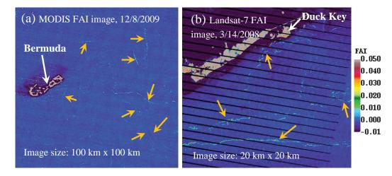
Figure 3.13 MODIS and Landsat FAI images (250- and 30-m resolutions, respectively) showing Sargassum-like features in the Sargasso Sea near Bermuda at 32.30°N, 64.77°W (a) and in the Florida Strait near Duck Key at 24.77°N 80.91°W (b). Some of the prominent features are annotated with brown arrows. Note that the slicks shown in (b) cannot be detected by MODIS on the same day due to the coarser resolution of MODIS.
