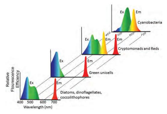
**Figure 2.4** General characteristics of fluorescence excitation (Ex) and emission (Em) spectra for various groups of phytoplankton. Phytoplankton taxa with phycobiliproteins (cyanobacteria, cryptomonads) have distinctive emission peaks compared to other groups. Excitation spectra exhibit more subtle variations according to photosynthetic accessory pigment composition. Modified from Yentsch and Phinney (1985).
