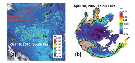
Figure 3.9 (a) MODIS-Aqua FAI image showing a *Trichodesmium* bloom south of Fiji Island in the South Pacific on 18 October 2010. The bloom showed spectral curvatures in the blue-green wavelengths similar to those shown in Fig. 3.8; (b) MODIS-Aqua FAI image showing a cyanobacteria bloom of *Microcystis* aeruginosa in Taihu Lake, China (a shallow, freshwater lake of about 2300 km<sup>2</sup> centered around 31.2°N, 120.2°E.
