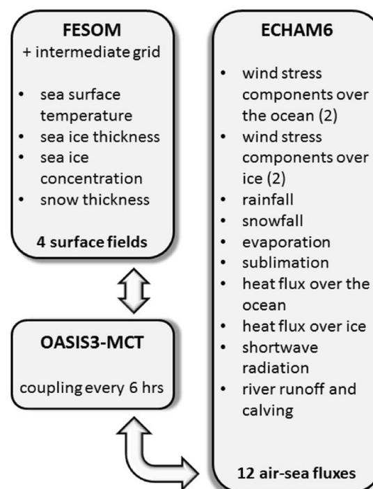
**Fig. 2** Schematic of the coupling procedure: ECHAM6 computes 12 air-sea fluxes based on 4 surface fields provided by FESOM. The 6-hourly averaged fields and 6-hourly accumulated fluxes are mapped between the model components every 6 h employing an intermediate exchange grid together with the OASIS3-MCT coupler
