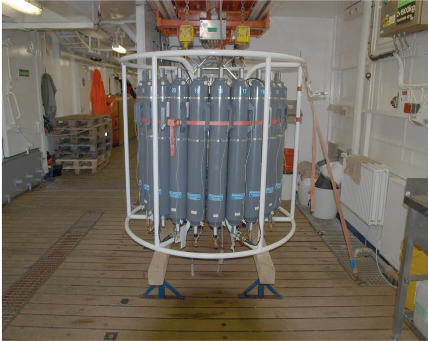
*Fig. 7.2: CTD/water sampler. The CTD with the pair of temperature/conductivity sensors are behind the samplers. The arrows indicated the shots and silicon tubes which were attached to the intake at each sensor pair. From the shots salt water was filled into the conductivity cell to prevent freezing. The shots were removed just before the CTD/water sampler goes overboard.*
