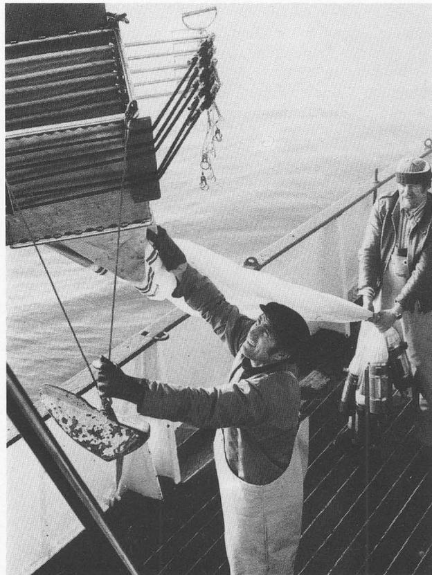
Sampling with the multiple opening and closing net on board FK „Alkor“ (photo: E. Mempel)
