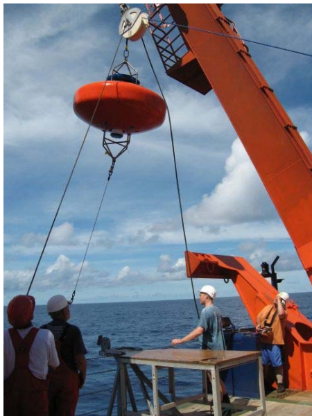
The top of current meter mooring is taken out. Inside the float an ADCP (Acoustic Doppler Current Profiler) is installed
