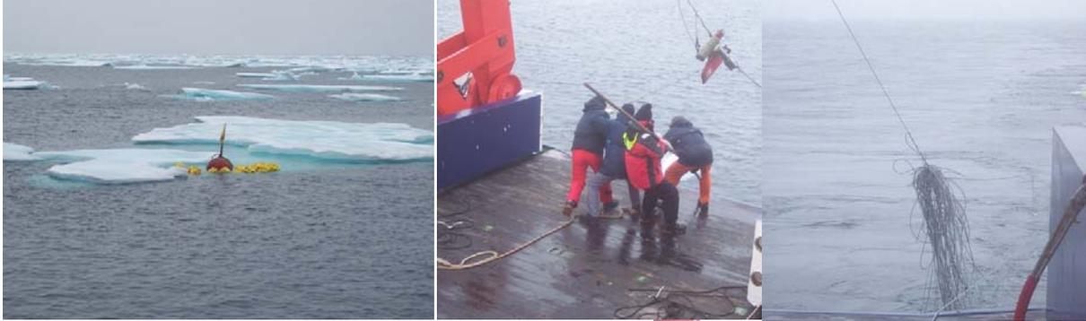
***Mooring A recovery:*** the mooring A is finally seen, embedded in a big growler (up left). The first currentmeter to come is the deepest one (up center), quickly followed by a mass of cables (right) and a huge ball of steel cable (up right).
