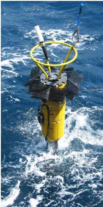
The 4<sup>th</sup> station is placed on the upper continental slope at 800m depth. Therefore, the favorable meteorological conditions give us an excellent opportunity to test our new Vertical Microstructure Profiler. Deployed at 14:35 local time, it pops up half an hour later, and is easily localized by both VHF and captain's eyes. After a very smooth approach, the VMP is recovered with the starboard crane without difficulty. 3 hydrological stations close this very active day.
