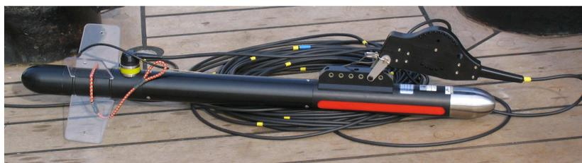
Figure 2.3: Side Scan Sonar
