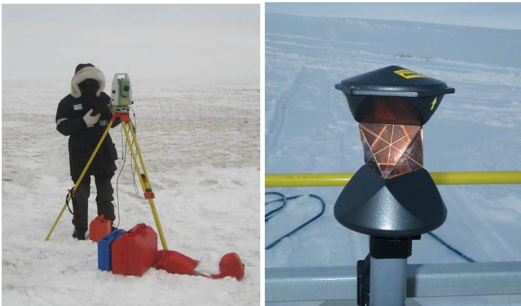
**Figure 6-1** Geodetic surveying equipment used for positioning: self-tracking total station (left) and prism (right).
