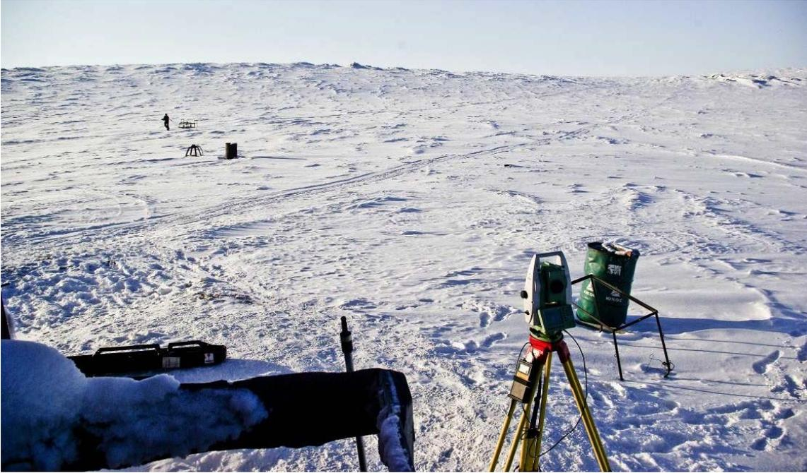
**Figure 7-4** Impression of GPR data acquisition on the western part of profile A1 (see Figure 7-5) in spring. The eastern part of the profile can be seen in foreground. Northernmost point of both profiles is located on the crest at the horizon.
