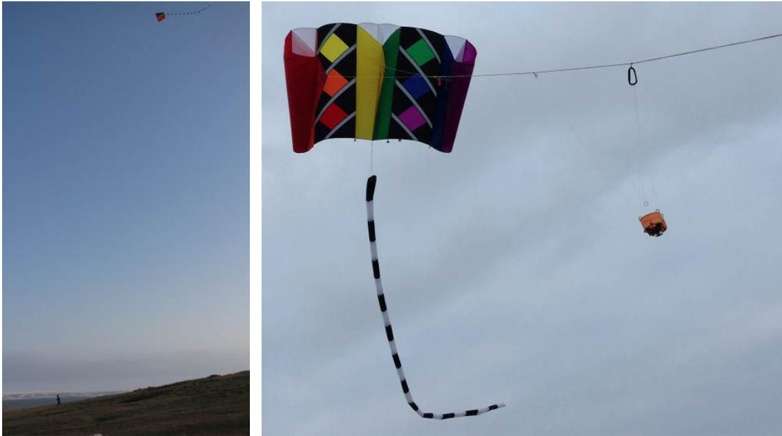
**Figure 6-2** Kite aerial photography system that was used as supplementary low-cost remote sensing tool. Left: Field impression of data acquisition. Right: Close up of kite and camera-equipped rig.
