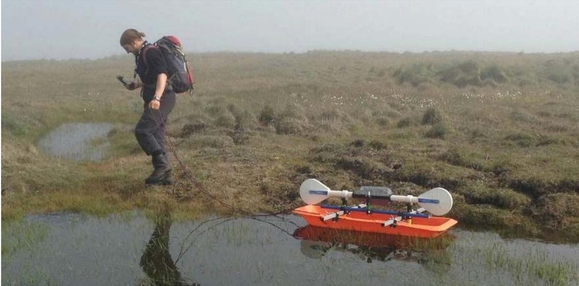
**Figure 7-2** Impression of EM data acquisition on Bol'shoy Lyakhovsky. The EMI device is mounted on a pulka and pulled across the survey site. A manually carried data logger triggers data acquisition with a constant time interval. Positioning is either performed by a self-tracking total station or with an internal GPS of the data logger.
