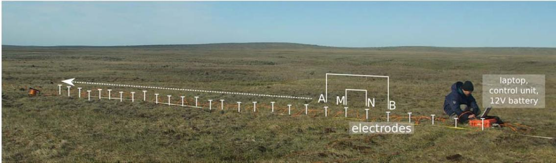
**Figure 7-3** Impression of ERT data acquisition on Bol'shoy Lyakhovsky. Our survey lines consist of 50 electrodes that are connected by a multi-core cable to a control unit with integrated power supply. A laptop is used for data acquisition.
