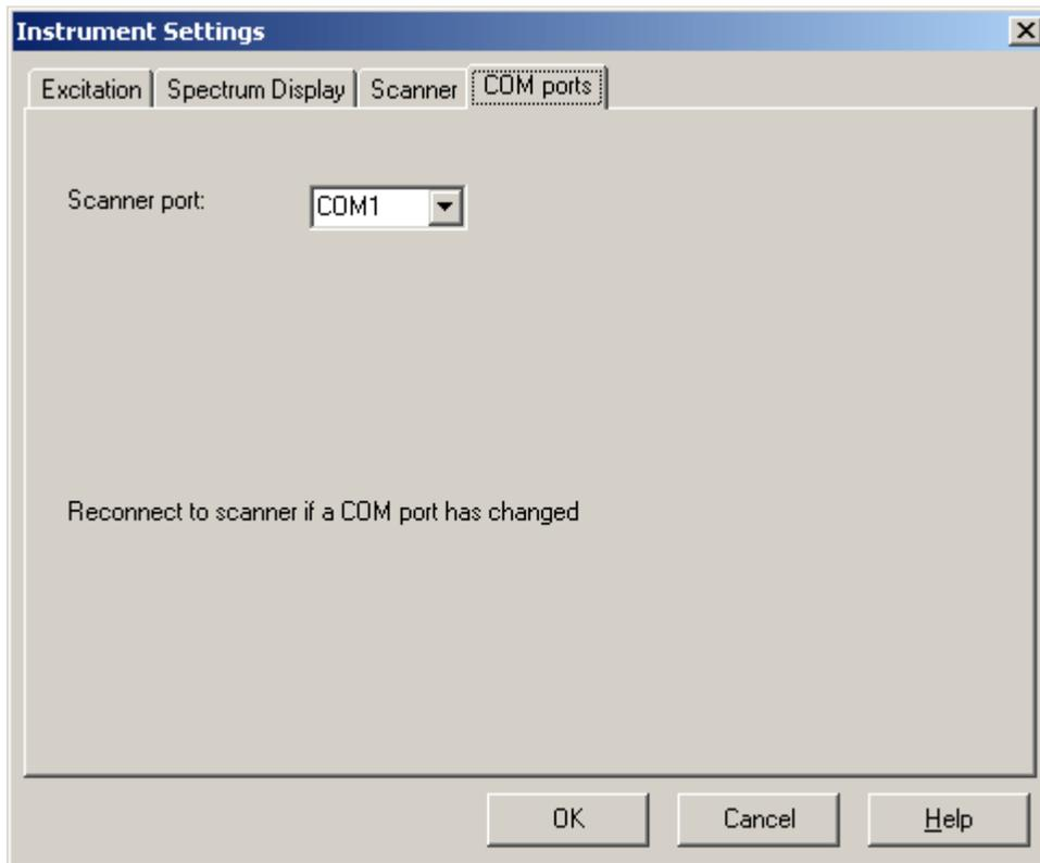
The scanner requires a serial COM port on the computer. The **Scanner port** setting determine which port number physically connects to the appropriate device. If a settings is changed the program should be re-connected to the scanner in order to activate the new settings.
