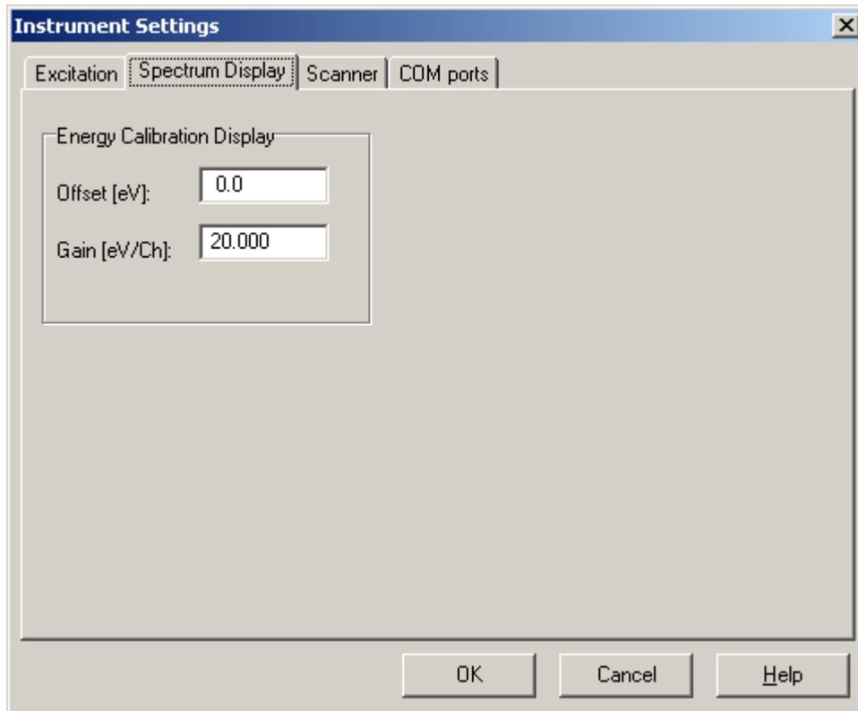
Both Energy Calibration settings **Offset** and **Gain** are implemented to transform the spectrum channel numbers, in the Spectrum Display Panel, into energy values. The settings on this screen are only to calculate the displayed energy value of the cursor in the Spectrum Display Panel. This energy value is displayed in the right corner of the statusbar.
