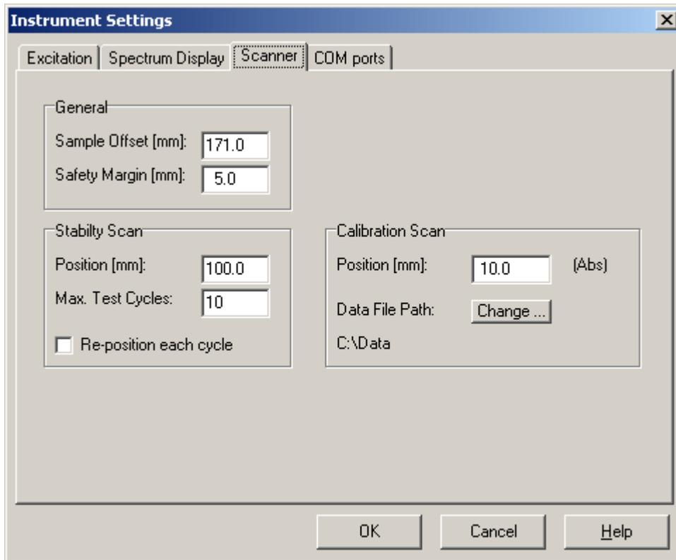
The General settings **Sample Offset** and **Safety Margin** are implemented to calibrate the scanners X-position and to prevent the scanner from measuring too close to the cores edges. The Sample Offset is the distance between the scanners homing-switch and the "0 cm" location of the core to be measured. Adjust this value if the mechanical "0 cm" position has been changed.
