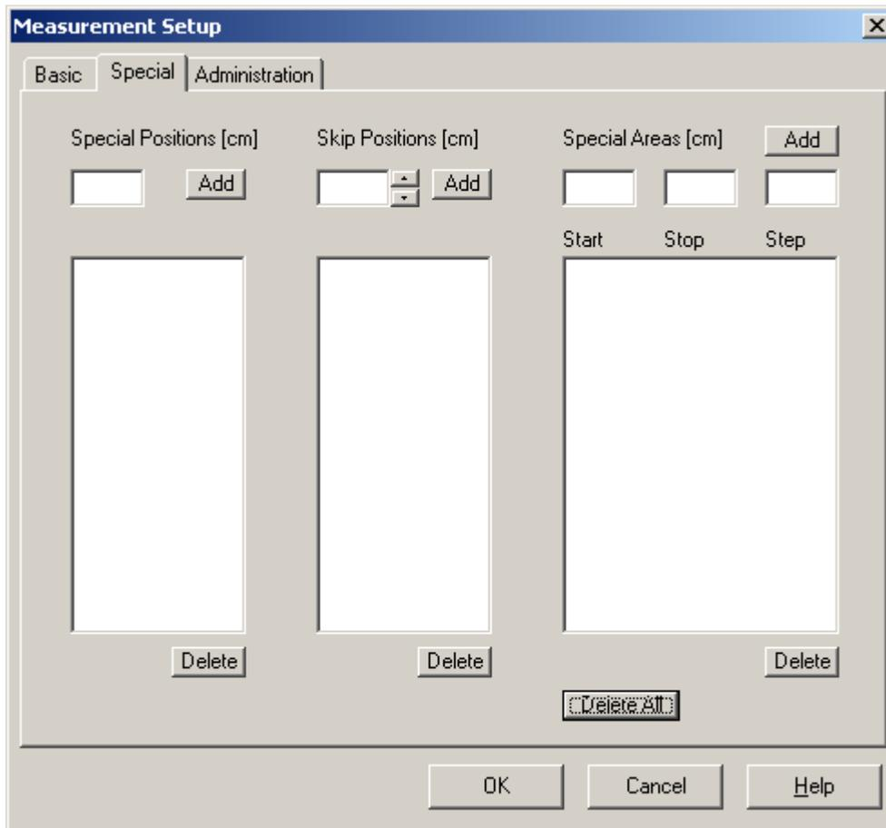
During a step scan the scanner jumps with Step Size steps over the core. To anticipate better on possible interesting core positions or huge gaps in the sediment surface it is possible to define **Special Positions** (e.g. in between a normal step), **Skip Positions** (a normal step that should be skipped) and **Special Areas** (a possible interesting area where one would like to step with a smaller step size).
