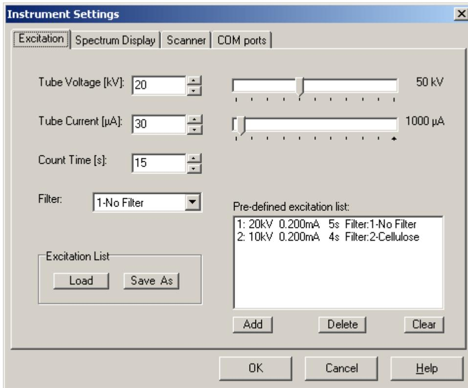
To set an X-Ray excitation condition adjust the **kV** and **mA** sliders with the left mouse button pressed at the correct value. Select the appropriate **CountTime(\*)** and **Filter** between X-Ray tube and sample.
