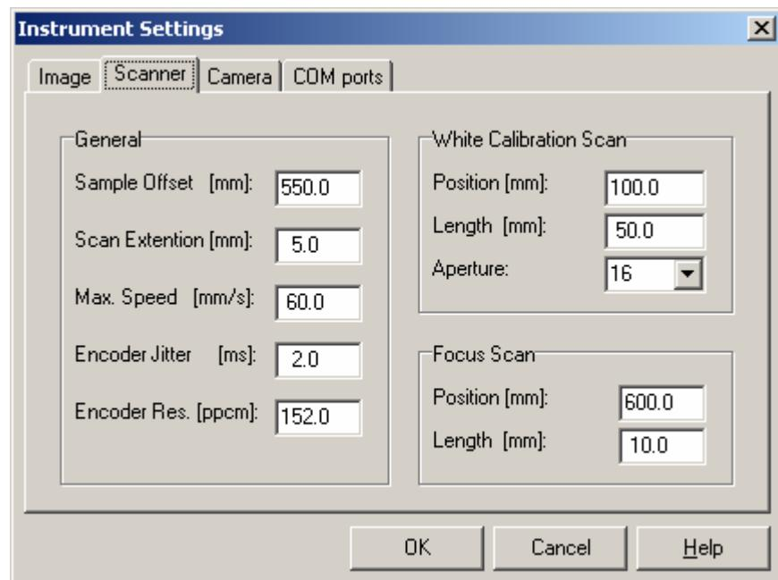
A general scanner setting is Sample Offset. This is the distance between the homing switch and the location where the sample is located. Before each line scan the camera and light source are positioned at this location.
