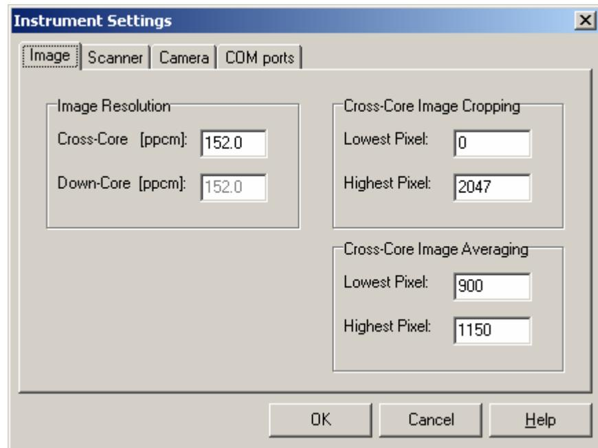
In order to know the exact size of the details on the image it is necessary to know the cross-core image resolution. The height of the camera above the sample and the lens type are important factors.
