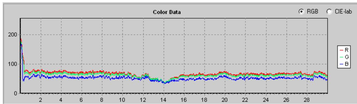
The color data that is automatically calculated at the end of a line scan is based on that part of the sample that is used for XRF analysis. The exact pixel numbers in cross-core and down-core direction can be adjusted on the Instrument Settings screen.
