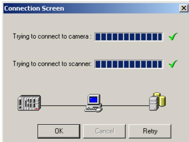
When the connection has been established the remaining toolbar buttons become active. The instrument settings button opens a window that contains the instrument related settings and the measurement setup button opens a window that contains the measurement related settings like sample name and length.
