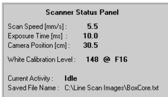
The Scan Speed depends on the camera Exposure Time and the down-core image resolution. The Camera Position is the actual position of the camera. The White
