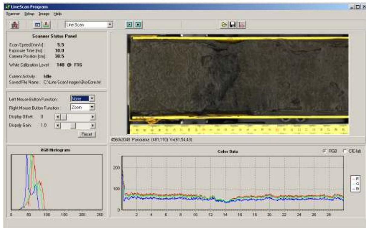
At the top of the window there is a menu and an application toolbar. On the left there are three panels. The upper panel shows the status of the camera system. The middle panel contains various mouse functions and image display controls. The lower panel shows the distribution of pixel intensities of a selected area of the image.
