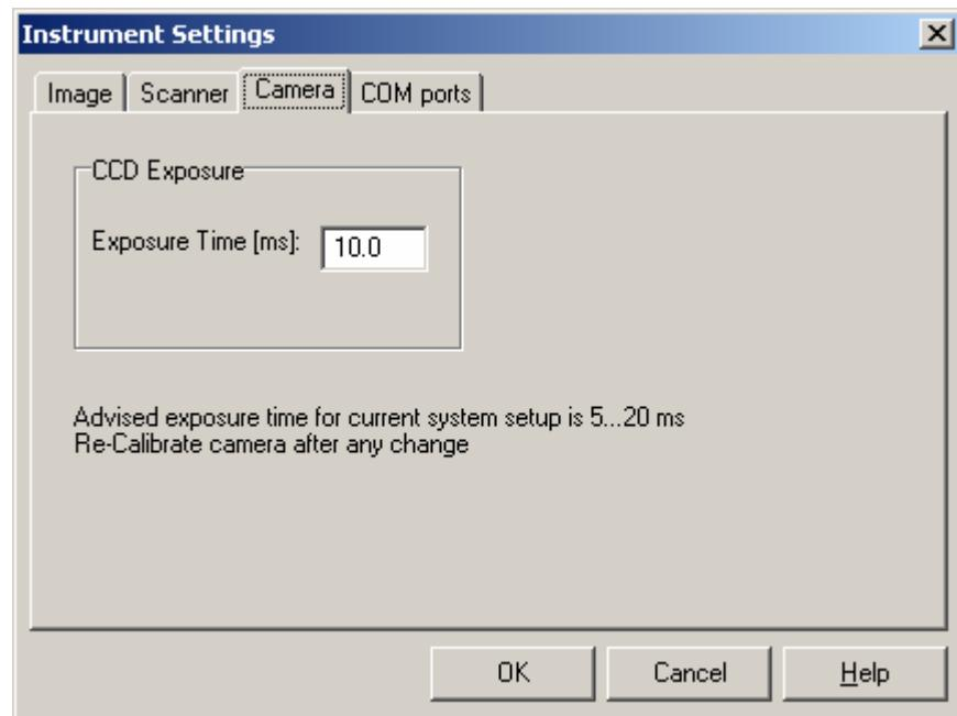
On the camera tab the camera Exposure Time can be set. The exposure time for each line is a critical parameter that controls the actual scan speed and the required aperture setting and therefore the field of depth.
