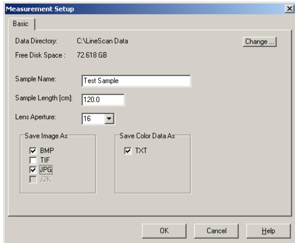
A color data file can easily be imported in MS Excel. Position, RGB and CIE-lab data becomes available. Also the down-core and cross-core image resolution as well as the pixel coordinates of the image area from which the color data was taken are available. Pixel (0,0) is the upper-left pixel of the image.
