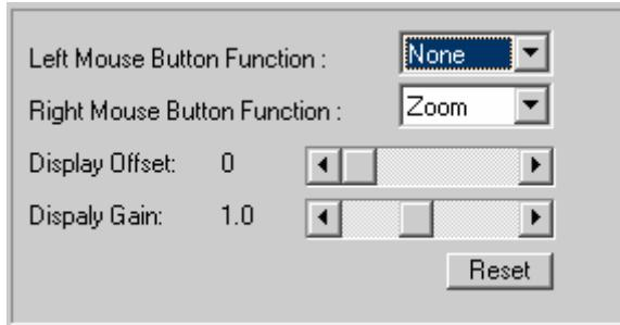
The left mouse button functions are :      None, Rubber, Frame, Area
