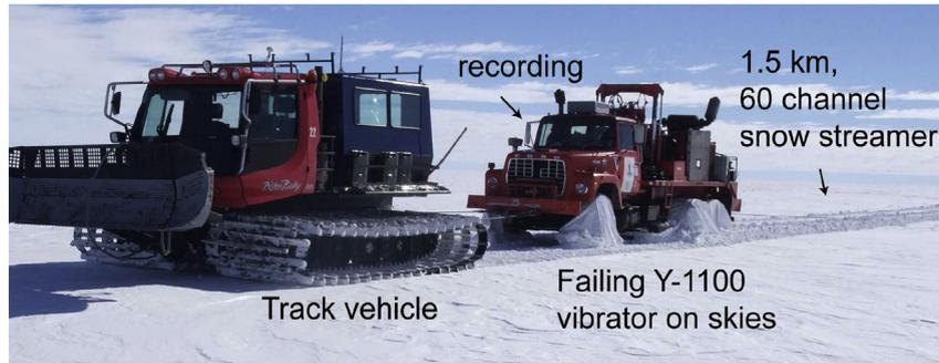
Fig. 2. Failing vibrator mounted on skis and pulled by a Pistenbully as used in 2010 and 2011 on Ekströmsen and Halvfarryggen. In 2011 the streamer was mounted to and pulled by the Failing truck. For wide-angle surveys, the streamer is pulled by a different vehicle, independently of the source.
