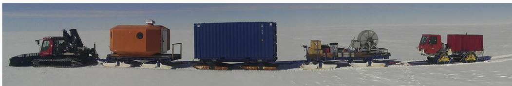
Fig. 4. Seismic train used in 2014 for the long-distance traverse on Ekströmsen and in its catchment. From left to right: Pistenbully Polar 300 pulling vehicle, living quarter, extended high-cube container set-up as EnviroVibe garage and workshop, freight sled with streamer winch, EnviroVibe on PE-sled. The streamer lead-in cable (white, far right) is guided to the front of the EnviroVibe and connected to the data acquisition units inside the operator's cabin.
