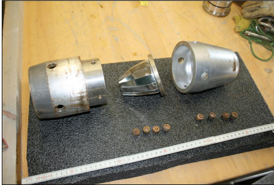
**Details of the Core Bit & Core Catcher**
