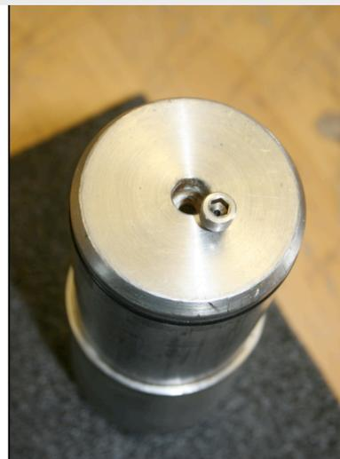
Lower side of upper piston with water-through-flow screw
