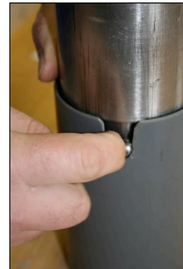
**Insertion of steel spheres**
