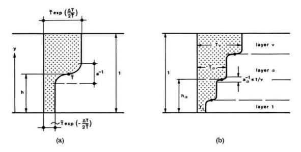
Fig. 2. Temperature distribution on a layer of thickness 1 according to equation (4.1), (a), and equation (4.2),(b)
