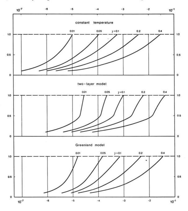
Fig. 11. Zeroth order velocity distribution for a single layer (top), the two layer model (middle) and the Greenland model (bottom), plotted for various inclination angles  $\gamma$ .
