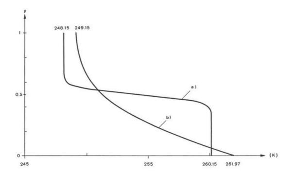
Fig. 3 Temperature distribution for the two layer model, (a), according to the temperature distribution (4.1) and for the Greenland model, (b), according to Robbin's formula (4.7).
