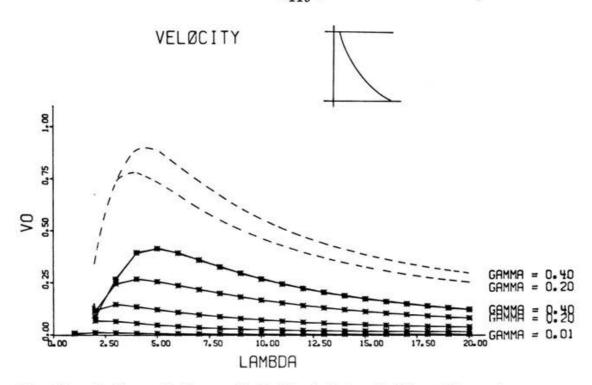
Fig. 13a. Surface velocity amplitude VO plotted against  $\lambda$  and for various values of  $\gamma$ . Plotted are also corresponding results for a layer with constant material properties.
