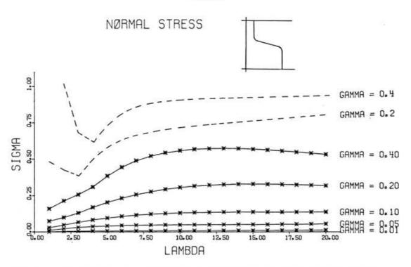
Fig. 9a. First order normal stress amplitude  $\Sigma$  for the two-layer model as a function of  $\lambda$  and for various inclination angles  $\gamma$ . Shown are also corresponding results for the single layer for  $\gamma$  = (0.2, 0.4). (dashed).
