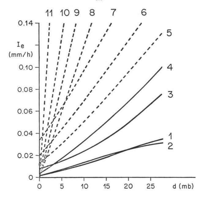
Fig. 2 Intensity of evaporation (I<sub>e</sub>) as a function of the average monthly air saturation deficit (d) for various gauges and precipitation forms. Liquid precipitation: 1 - Polish standard gauge, 2 - Hellmann gauge, 3 - Hungarian standard gauge, 4 -, 5 -, 6 -, 7 - Tretyakov gauge and wind speed at the level of the gauge rim 0-2, 2-4, 4-6 and 6-8 m/sec, respectively. Solid precipitation: 8 -, 9 -, 10 -, 11 - Tretyakov gauge and wind speed 0-2, 2-4, 4-6 and 6-8 m/sec, respectively.
