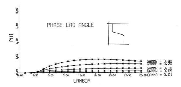
$\frac{\text{Fig. 7b.}}{\text{as a function of}} \ \, \varphi_{\text{T}} \ \, \text{for the shear stresses of the two layer model} \\ \text{as a function of} \ \, \lambda \ \, \text{and parameterized for various inclination} \\ \text{angles} \ \, \gamma \, .$
