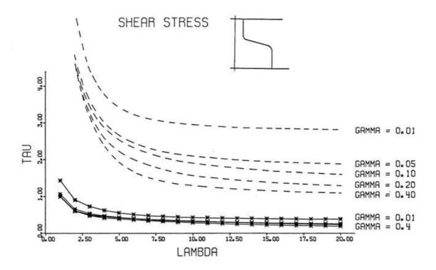
Fig. 7a . First order shear stress amplitude  $\odot$  for the two layer model as a function of  $\lambda$  and parametrized for various inclination angles  $\gamma$ . Shown is also the result for a one-layer model.
