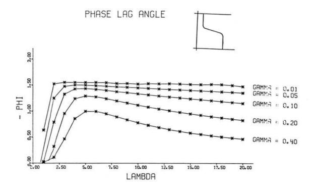
Fig. 6. Phase lag angle of the two layer model corresponding to the filter function F plotted against wave length  $\lambda$  and parameterized for various inclination angles  $\gamma$ .
