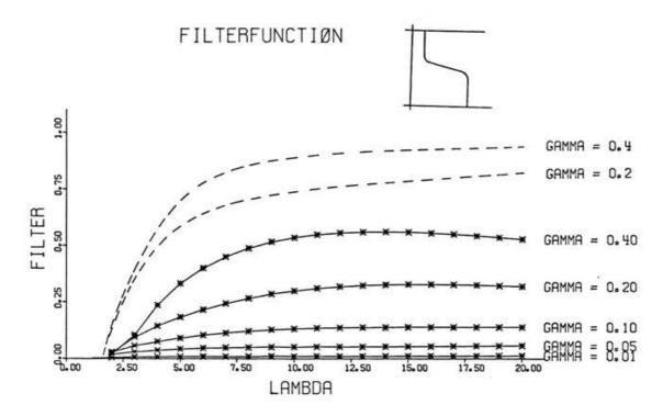
Fig. 4 Filter function of the layer model characterising the transfer of bottom undulations to the surface as a function of wave length  $\lambda$  and parameterized for various inclination angles  $\gamma$ . Shown are also the curves  $\gamma = (0.4, 0.2)$  for the one layer model (dashed).
