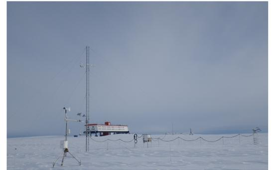
AWS setup next to Neumayer meteorological mast for comparison experiment in 2011. Photo: Jölund Asseng (AWI)
