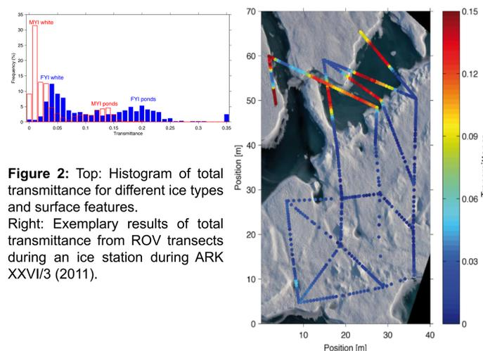
**Figure 2:** Top: Histogram of total transmittance for different ice types and surface features. Right: Exemplary results of total transmittance from ROV transects during an ice station during ARK XXVI/3 (2011).
