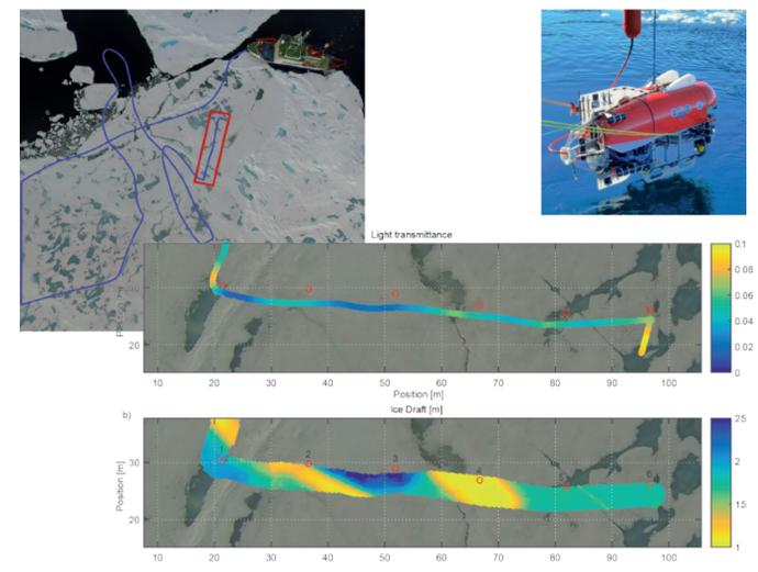
**Figure 3:** Top left: Aerial photograph with the dive track (red box). Polarstern is anchored to the ice floe (top right corner). Top right: Photograph of the NUI hybrid-ROV, which was used to obtain these results. Bottom: Exemplary light transmittance and sea ice thickness along the dive track (PS92, 2015).
