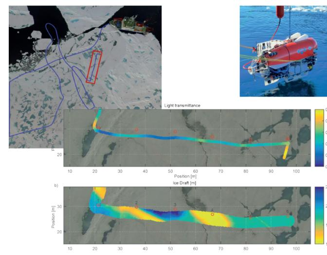
**Figure 3:** Top left: Aerial photograph with the dive track (red box). Top right: Photograph of the NUI hybrid-ROV, which was used to obtain these results. Bottom: Exemplary light transmittance and sea ice thickness along the dive track (PS92, 2015).
