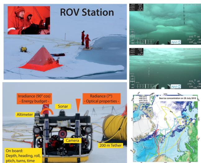
**Figure 1:** Left: Set up and instrumentation for under-ice transects of spectral radiation using a Remotely Operated Vehicle (ROV) operated directly from the sea ice, photographs taken by the ROV. Marker length: 1 m. Right bottom: Cruise tracks of all field measurements.
