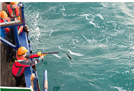
Fig.2: First measurement from a moving vessel. The XBT is employed. Photo: Michael Ginzburg, AWI (Photo: Alfred Wegener Institut)
