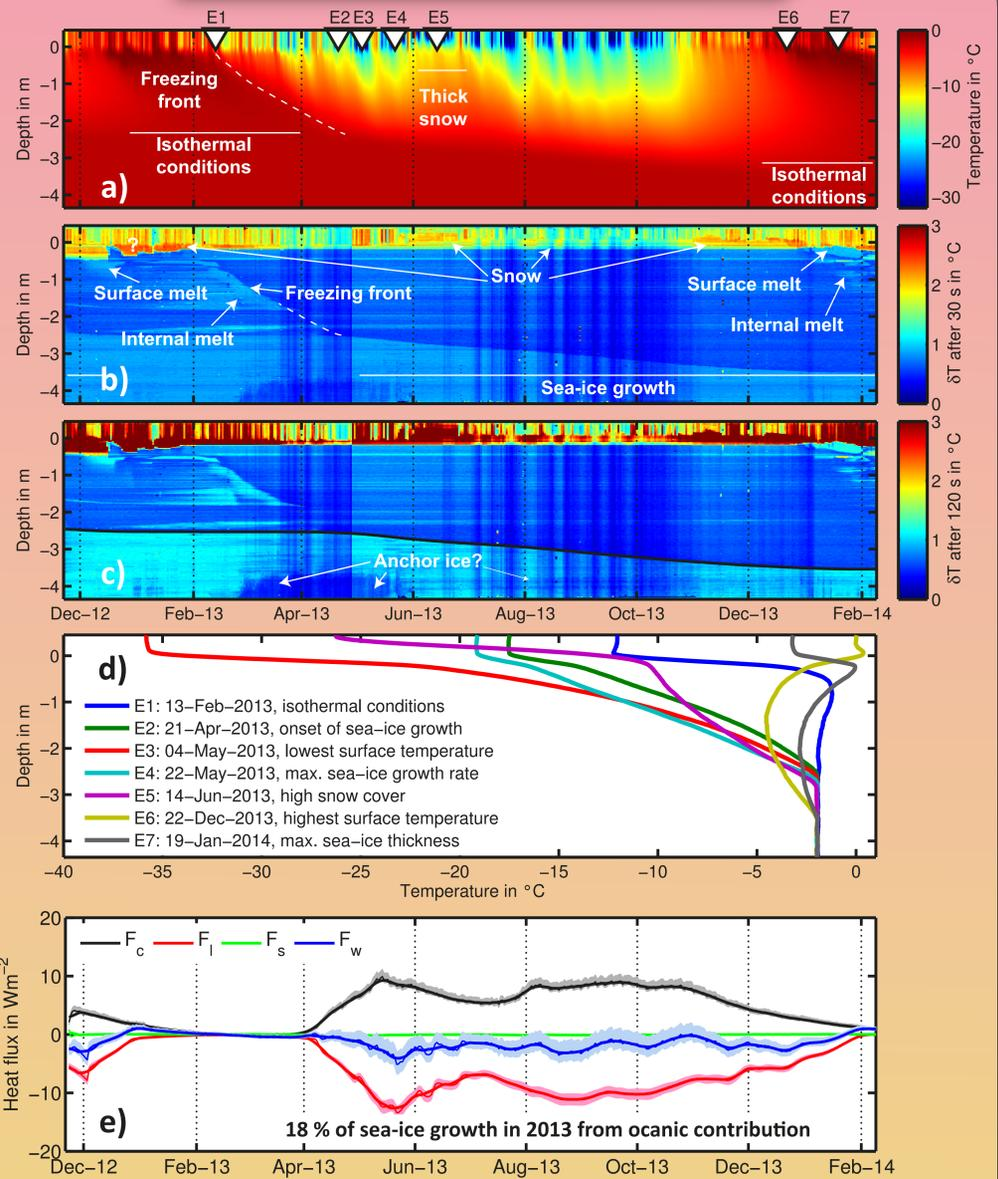
a) Thermistor chain daily temperature profiles, b) temperature rise after 30 s of heating, c) temperature rise after 120 s of heating, d) selected characteristic temperature profiles, e) basal energy budget ( $F_c$ : conductive,  $F_l$ : latent,  $F_s$ : sensible,  $F_w$ : residual heat flux. The shaded areas represent the cumulative individual measurement uncertainties. Upward heat fluxes, warming and melting have positive sign.)
