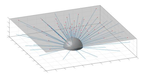
**Figure 1:** Geometry of the light model integrator. The half sphere represents the unit Lebedev sphere with blue rays pointing in the direction of each segment. Rays are intersecting the surface (grey transparent layer) in the location of the red dots. At these locations radiance values are taken from the inhomogenous surface matrix.
