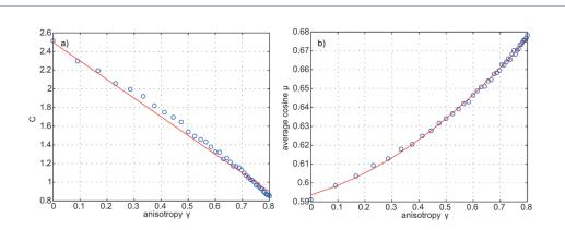
Figure 5. (a) The ratio of irradiance and radiance (C value) observed underneath the sea ice as a function of the anisotropy of the scattering coefficient  $\gamma$ . Blue circles show the results of Monte Carlo simulations, while the red line depicts the suggested parameterization  $C = 2.5 - 2\gamma$ . (b) Average cosine underneath the sea ice as a function of anisotropy  $\gamma$ .
