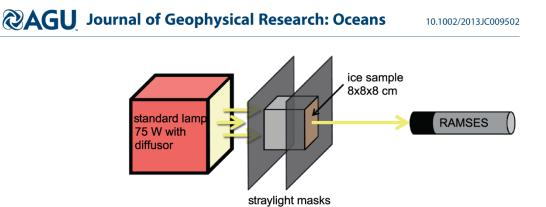
Figure 2. Sketch of the experimental setup to measure horizontal and vertical light extinction.
