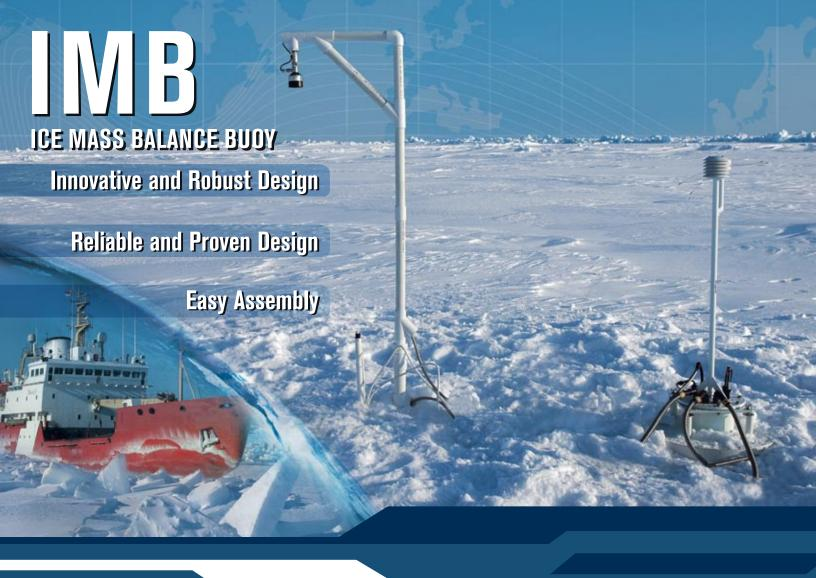
The METOCEAN Ice Mass Balance Buoy was developed in partnership with CRREL (Cold Regions Research and Engineering Laboratory). The Ice Mass Balance Buoy instrumentation is used to measure ice thickness, ice temperature, and to acquire meteorological and upper oceanographic data.
