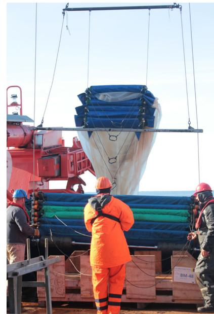
Abb. 1.4: Das RMT as it is being hauled in. All nets are closed. (@ Fokje Schaafsma)
