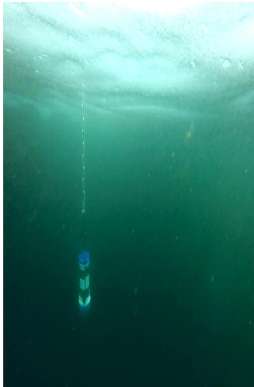
*Fig. 4.4: The ADCP under the ice (Photo, B. Juhls)*
