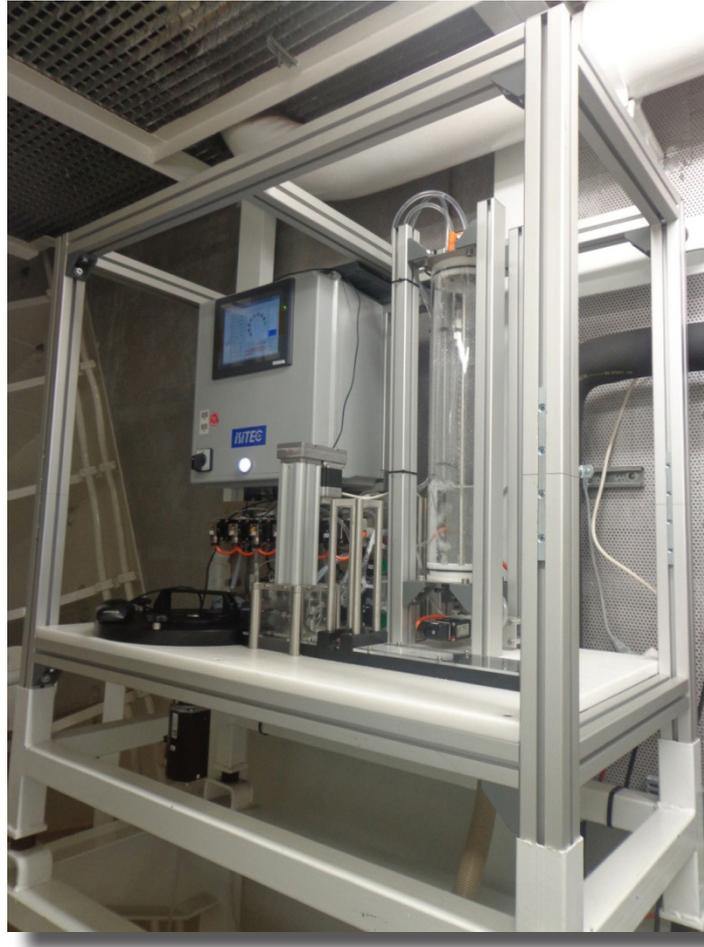
*Fig. 9.2.1: Automatic filtration system for marine microbes (AutoFiM) Sample reservoir could be filled with up to 5L of seawater. Filters are provided in a filter magazine and automatically placed under the filtration unit. When filtration is finished, generated filters are preserved with lysis buffer and stored in a rondell. Filtration operation is performed automatically*
