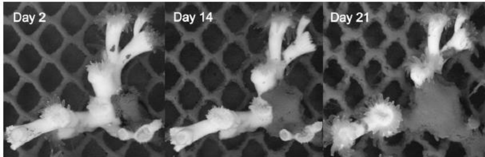
Fig. 6. Example of polyps and tissue smothered by accumulated drill cuttings. The total sediment load was 19 mm added in portions during 3 weeks.
