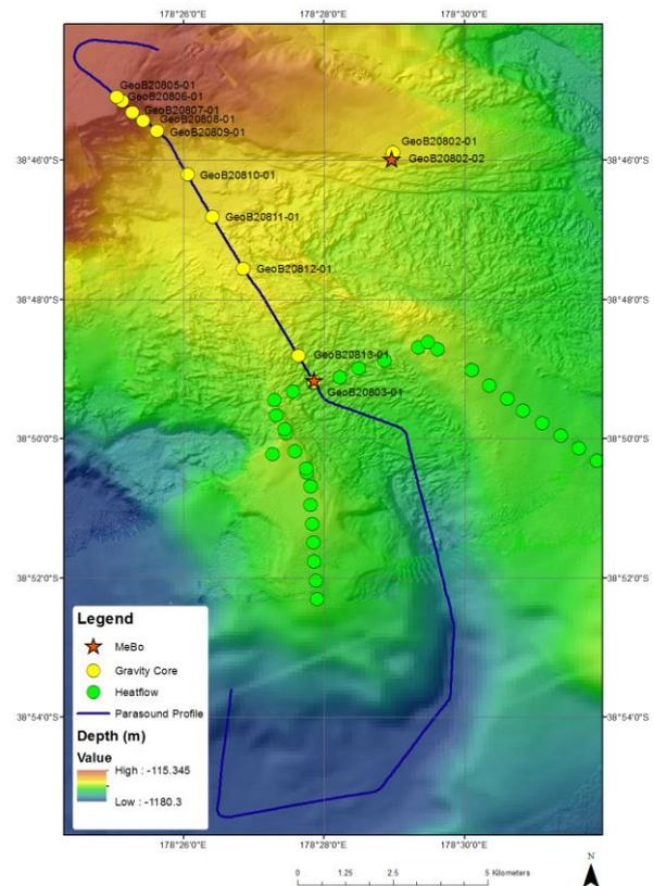
*Fig. 2 shows the Tuaheni working area with positions of already recovered gravity and MeBo cores as well as locations of heat flow measurements.*
