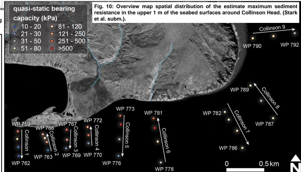
Fig. 10: Overview map spatial distribution of the estimate maximum sediment resistance in the upper 1 m of the seabed surfaces around Collinson Head. (Stark et al. subm.).
