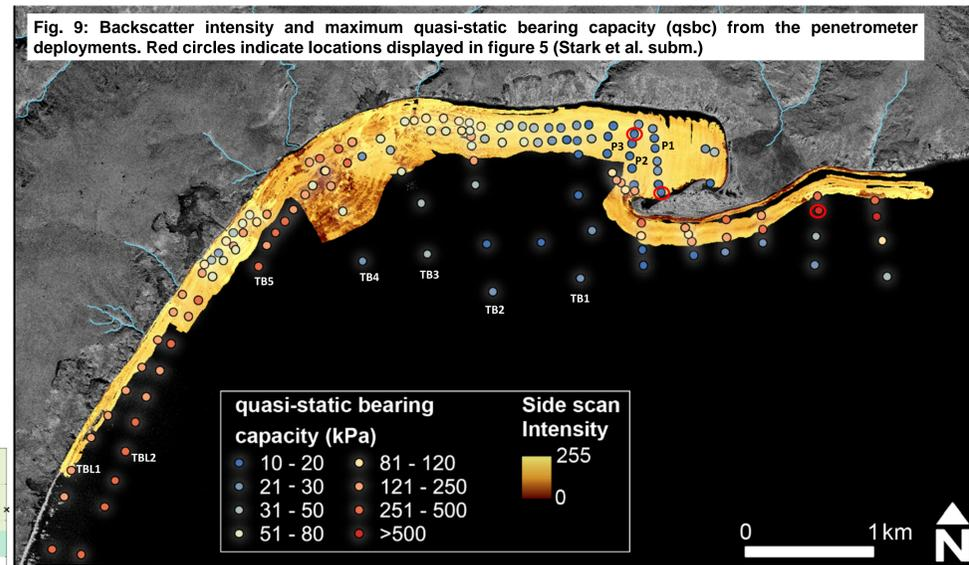
Fig. 9: Backscatter intensity and maximum quasi-static bearing capacity (qsbc) from the penetrometer deployments. Red circles indicate locations displayed in figure 5 (Stark et al. subm.).
