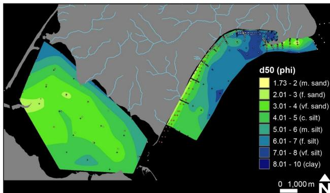
Fig. 6: Sediment map. Grab sample locations are indicated as black crosses, and *BlueDrop* deployments as circles (Stark et al. subm.).
