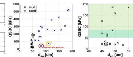
Fig. 8: Estimates of max. quasi-static bearing capacity (qsbc) vs.  $d_{50}$  (Stark et al. subm.).
