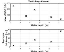
Fig. 7: Max. qsbcc and top layer thickness (Stark et al. subm.).
