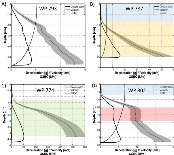
Fig. 5: *BlueDrop* penetrometer signatures from four exemplary locations. Different shadings indicated different geotechnical responses and sediment resistances to the penetration of the probe (Stark et al. subm.).
