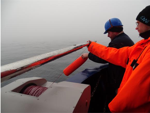
*Figure 5 : Attaching the protection foam on the UCTD line (photo credit : Amélie Bouchat)*
