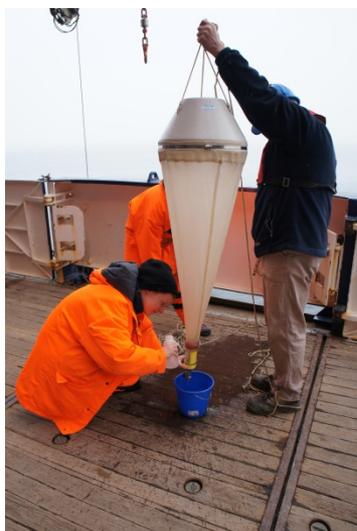
*Fig. 5: Hand net sampling. (Photo: T. Breckenfelder)*
