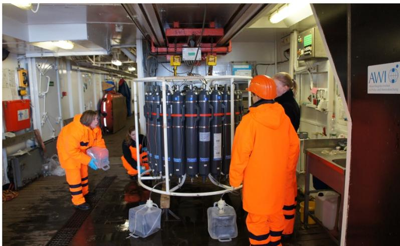
*Fig. 4: Water sampling for  $\delta^{13}\text{C}$ ,  $\delta^{18}\text{O}$ , nutrients, Nd and Hf analysis. (Photo: A. Krandick)*
