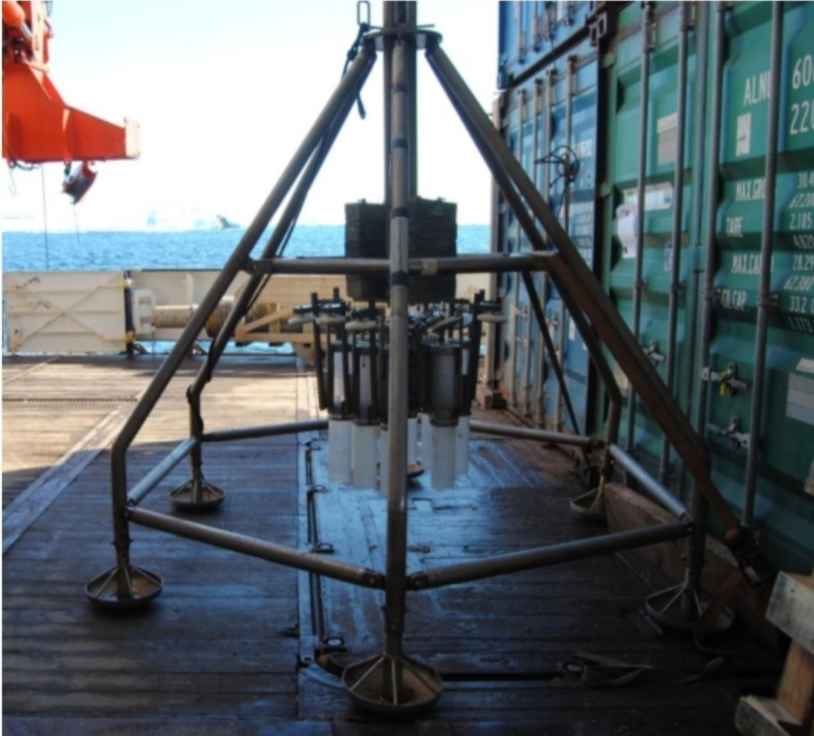
Figure 8: The multi-corer awaiting deployment on the working deck. Photo credit: Kirstin Werner
