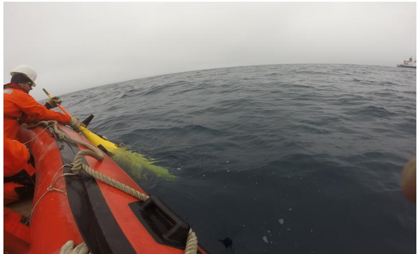
*Figure 7 : The insertion of the ocean glider into the water. Polarstern can be seen in the background (photo credit : James Williams)*
