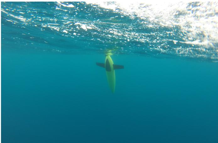
*Figure 8 : The ocean glider seen from underwater awaiting the dive command from its controllers in Bremerhaven (photo credit : James Williams)*
