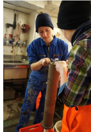
*Fig. 8: Cutting the multi corer in 1 cm thin layers. (Photo: K. Kretschmer)*
