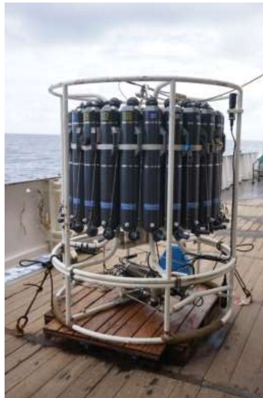
Figure 1: Rosette with mounted CTD probe. Photo: B. Springer.
