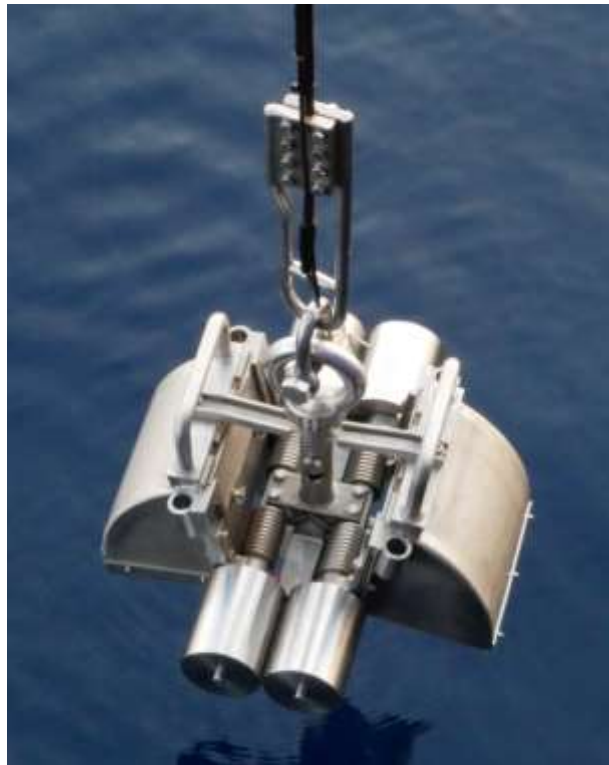
Figure 2: The Henning-grab is deployed. Foto: A. Ostmann.
