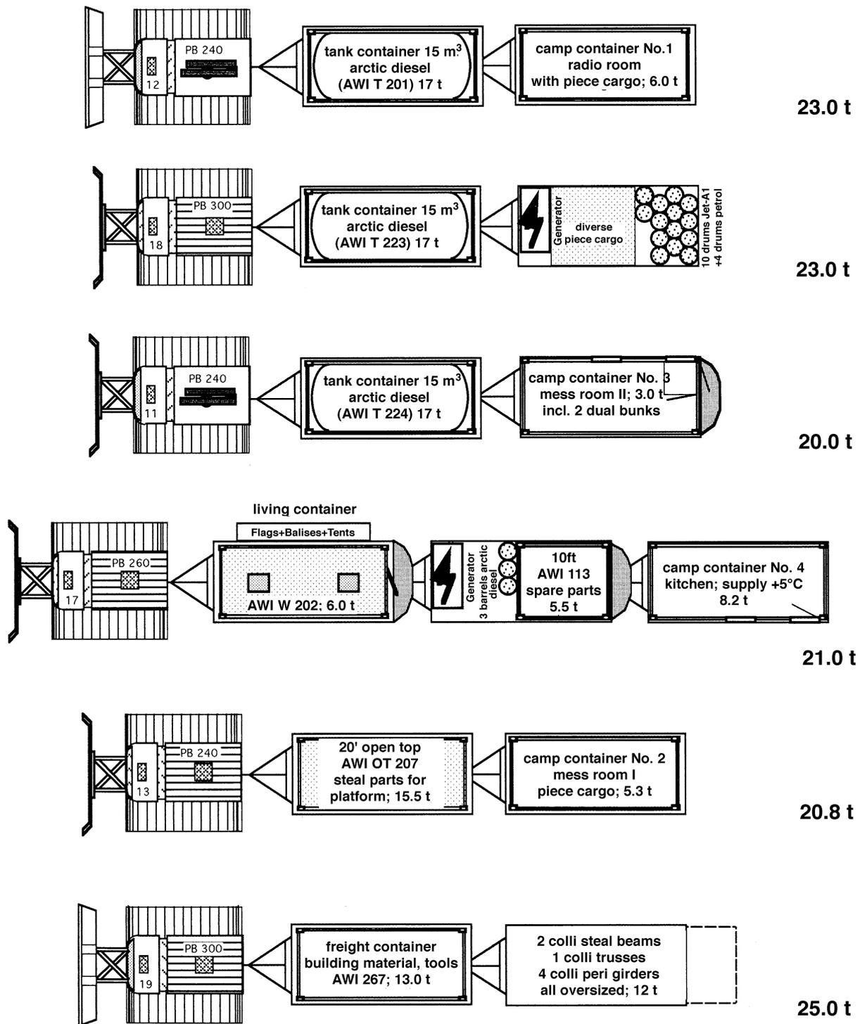
Fig. 2: Load plan for the first traverse of the 1999/2000 season ex Neumayer base to Kohlen base. The given weights illustrate the typical payload of about 20 t per sledge train..
