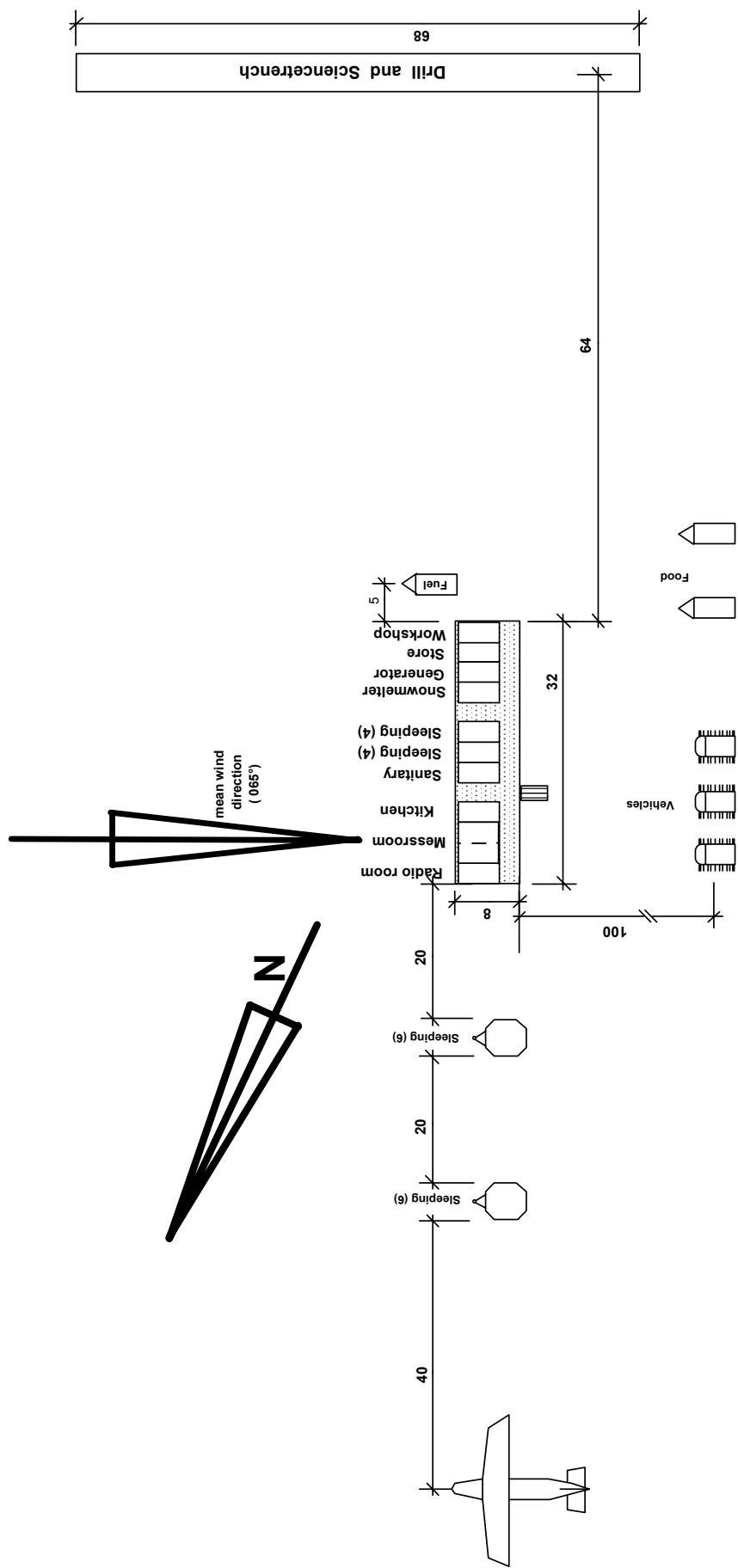
Fig. 4: The layout of Kohnen base. Distances in m.
