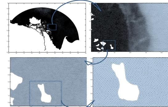
The unstructured grid for the considered domain. Element edge sizes vary from 30m to 850m. The grid contains 507875 nodes
