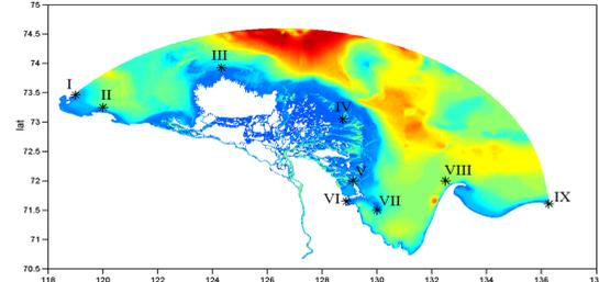
Reconstructed bathymetry for the Lena delta region, [m]. The negative values indicate the topography data above see level, the asterisks show the location of the stations used for validation of the tidal dynamics
