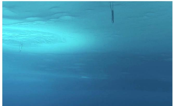
**Figure 6.2:** Under-ice measurements of radiative fluxes with fiber-optic detectors under level sea ice with varying snow/pond cover accounting for differences in light availability visible in the photograph.
