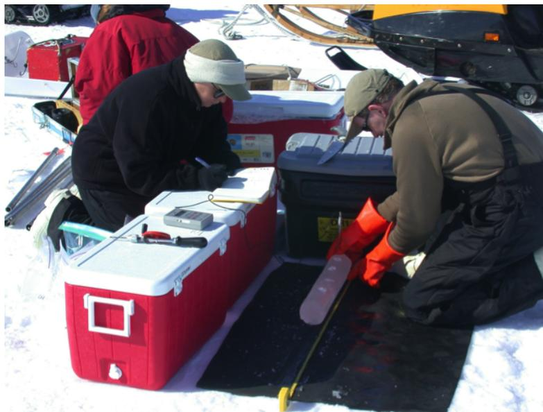
**Figure 5.1:** Extraction of an ice core with a gasoline-powered engine and a fiberglass-barrel corer (left). Field site (right), showing hand drill and thermometer for ice-core temperature measurements on top of the sample cooler at left and core laid out in the shade for processing.
