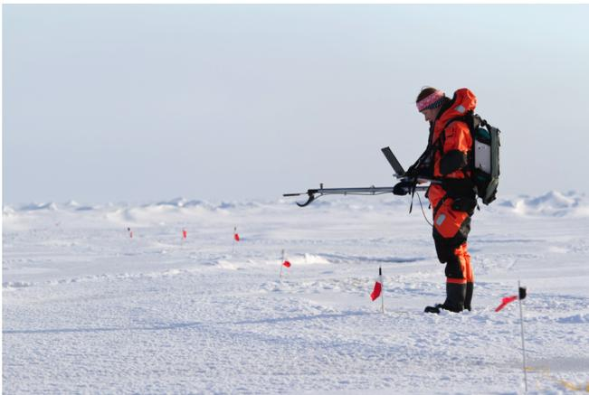
**Figure 6.1:** Surface-based measurement with a spectroradiometer (consisting of diffuser plate and fiber-optic detector at end of boom, laptop computer and back-pack with the radiometer).
