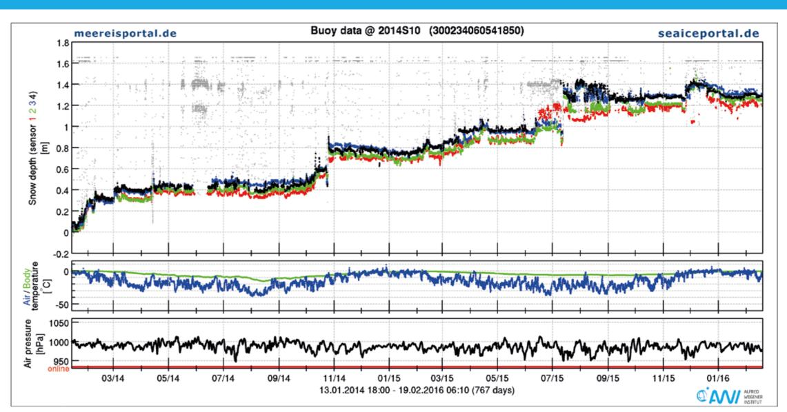
Results from snow buoy 2014S10, drifting through the Weddell Sea and reporting data for more than 2 years. Total snow accumulation is >1.2 m.
