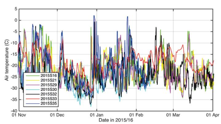
Air temperature (hourly, top) and snow depth (daily mean, right) from snow buoys on Arctic sea ice during winter 2015/16. Drift tracks are shown in the map above.
