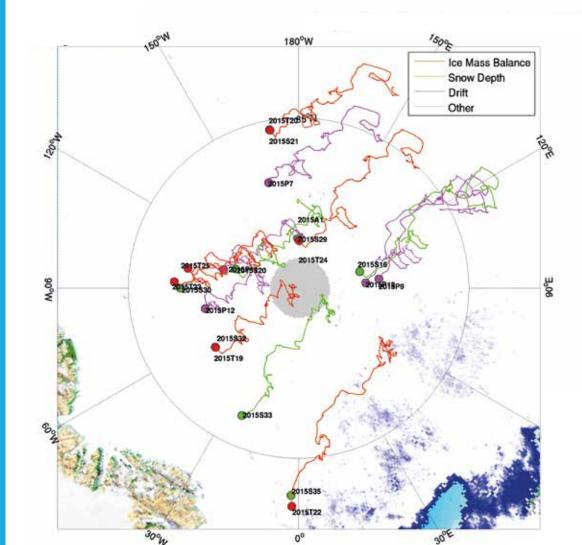
Snow buoys (green lines) contribute to a network of autonomous platforms in the Arctic (deployed in autumn 2015). (Figure: www.seaiceportal.de)
