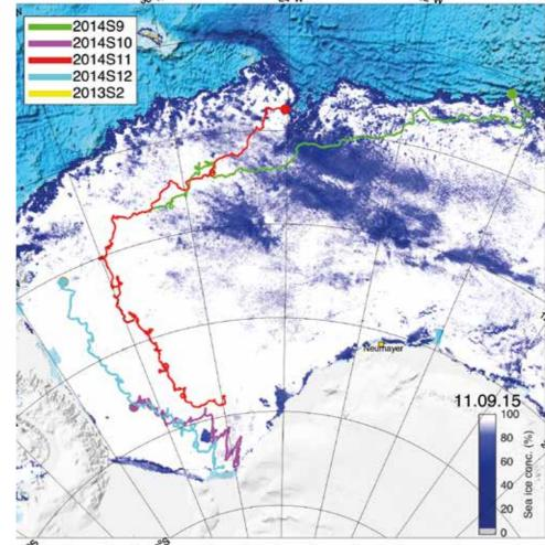
Four snow buoys drifting through the Weddell Sea. See also results **Section.** (Figure: www.seaiceportal.de)
